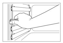
Pull the telescopic runners from the rear side of the wall and remove the telescopic runners.
